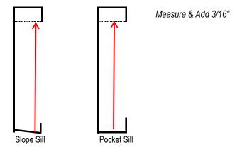
Measure from where the screen will rest on the sill of the window up to the <u>opening</u> of the top screen track, then add 3/16". For a deeper top track, you may be able to add 1/4".
